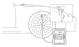
• Press the power button to start inflating. Do not touch the air hose during operation.
